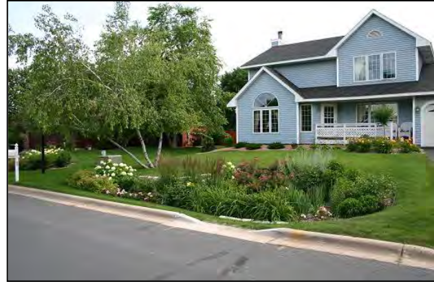
Residential Rain Garden
