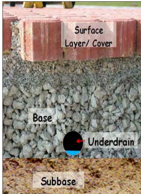
Typical Permeable Pavement System (Source: Hunt and Collins, 2008)
