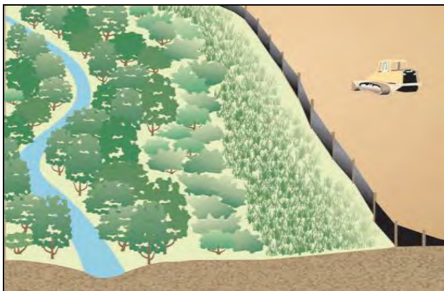
Silt Fence Used on a Construction Site
